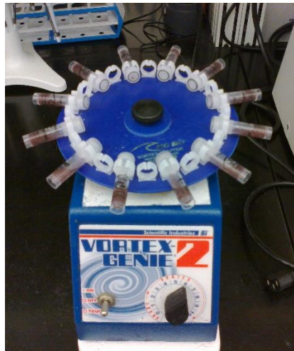
Fig. 2 The positions of bead tubes on the Vortex.
